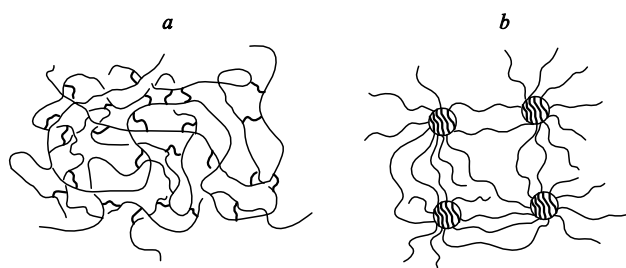
Figure 18. A scheme of a topological structure of polydimethylsiloxane networks cross-linked by a short-chain cross-linking agent. (a) the formation of bimodal networks according to Sharaf and Mark; 60 (b) the topological structure of the same network in the case of microphase separation.
